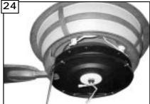
Check the motor for plastic shipping stabilizer tabs and remove them if they are present. The screws, washers, and motor pads are pre-installed to the blade brackets. Attach blade assembly to motor and tighten screws securely.
